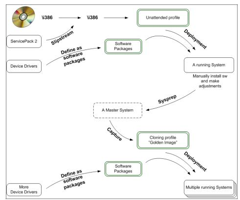
Figure 1-2 The main processes for a Windows XP mass distribution
